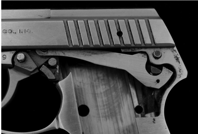
Figure 4.10 Close-up of an L.W. Seekamp pistol, showing the draw bar, which is connected to the trigger and the hammer strut. Just behind the trigger is the magazine safety lever, which disables the firing train when no magazine is inserted. (Image from author’s collection.)
